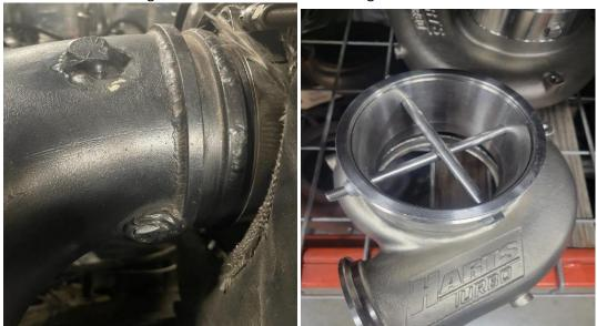
Pro Stock Tractors & Hot Rod Semi will be permitted to utilize turbocharger manufacturer's billet cage (without modification).
